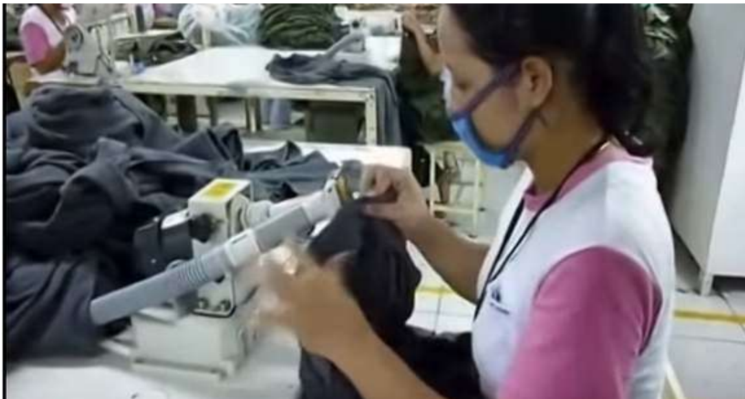
Fig1.3: Thread trimming machine
